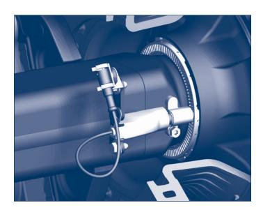
Almost all BPW axles can be retrofitted with ABS without problems. To do this, simply take the exciter ring, sensor brackets, sensors and fastening parts contained in the retrofit kit and attach them to the axle in accordance with the supplied installation drawing, then connect them to the vehicle electronic system.
