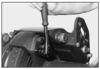
5. Lift the caliper away from the disc.
